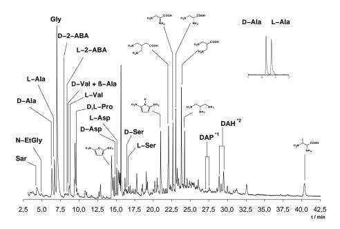
Figure 2.13: Gas chromatogram showing the amino acids and other compounds generated under simulated interstellar conditions by Muñoz-Caro et al.
