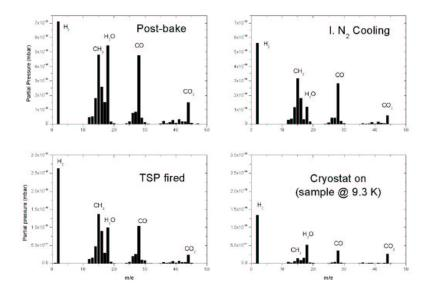
Figure 2.14: Top left: high vacuum conditions, comparable to those in all previous ice experiments in the Sackler laboratory. Top right, the vacuum conditions under ultra high vacuum conditions. Notice that the vacuum is now dominated by  $H_2$  and not  $H_2O$  molecules. Bottom left: the vacuum after sublimation pumping. Bottom right: system is cooled to 10 K, mimicking closest the interstellar conditions.
