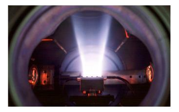
Figure 2.5: A planar plasma jet in full operation: a mixture of  $C_2H_2$  in He is discharged. Exotic species, such as the astrophysically relevant  $C_6H$ , are formed in the adiabatic expansion by recombination collisions. Typical rotational temperatures are 10 K.
