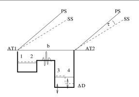
Figure 2.6: The interferometric principle of measuring the star separation  $\tau$  with PRIMA: the two telescopes AT1 and AT2, a baseline length *b* apart, receive light from the two off-axis stars, the primary star (PS) and the secondary star (SS), separated by  $\tau$ . Adjustment of one of the two Main Delay Lines and one of the four Differential Delay Lines (arrows) within the coherence length creates K band fringes on two detectors in the VLTI laboratory.
