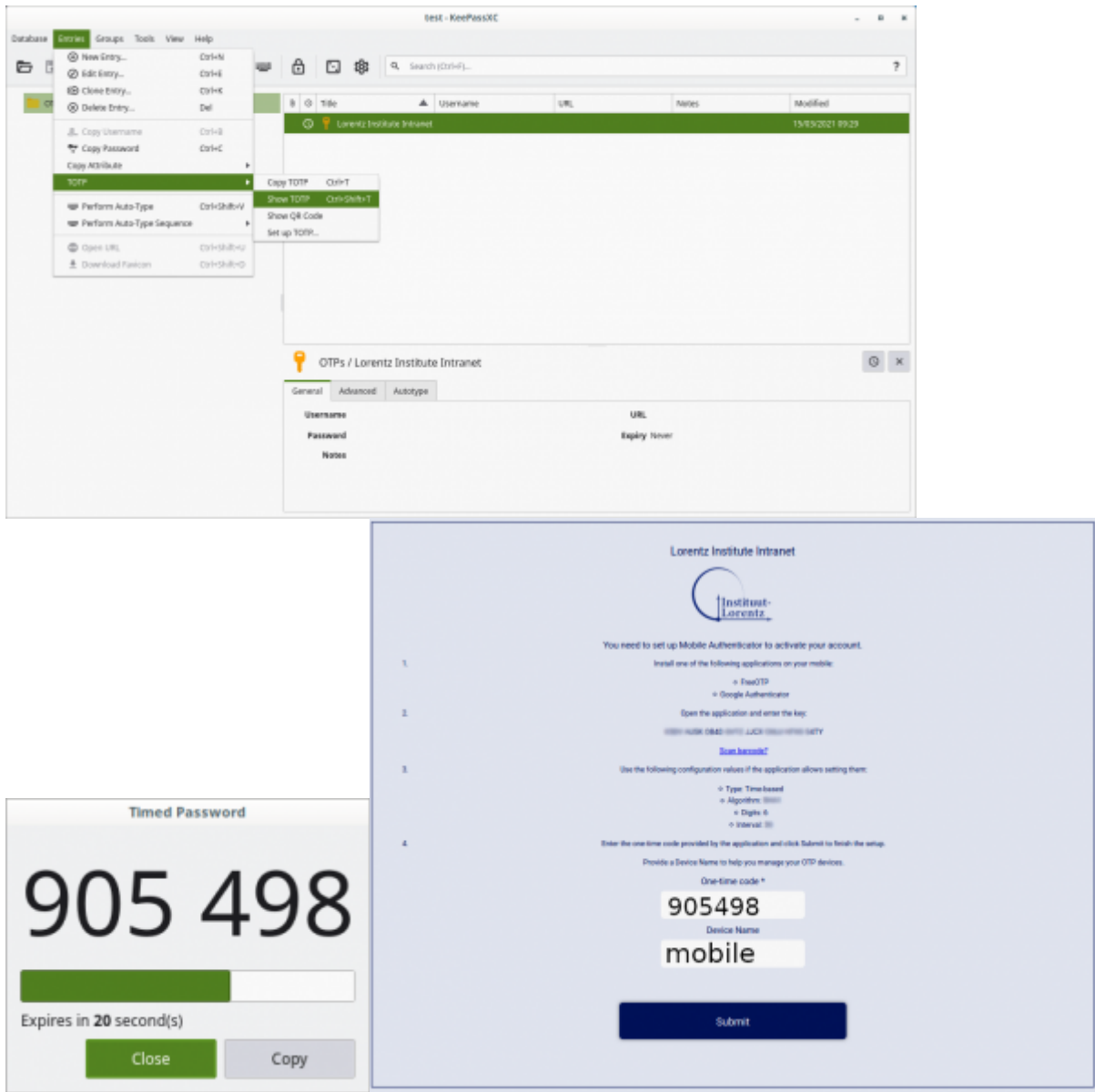
Figure 4: TOTP generation KeePassXC and final 2FA setup on the Lorentz Institute Identity Provider
