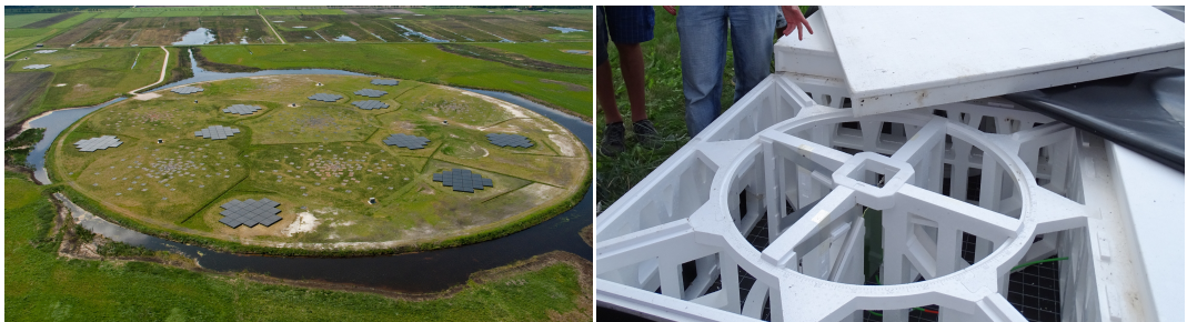
Figure 7.16: Left : LOFAR's so-called superterp located in Exloo, Drenthe in The Netherlands. The black tiles are the HBA antennas. The gray squares are the platforms of the LBA antennas. Right : a close-up of one of the HBA tiles, revealing the actual antennas suspended in styrofoam. Image credit: LOFAR / ASTRON (left); B. Wolba (right).
