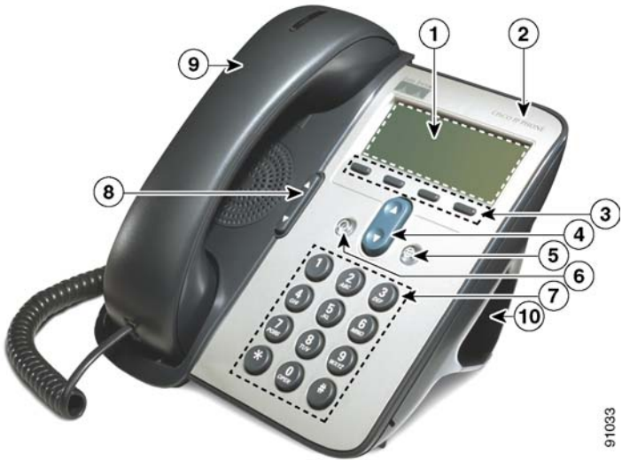
Figure 3 Cisco IP Phone 7912G Features
