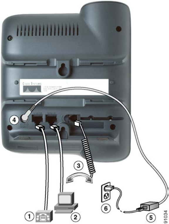
Figure 1 Cisco IP Phone 7912G Cable Connections
